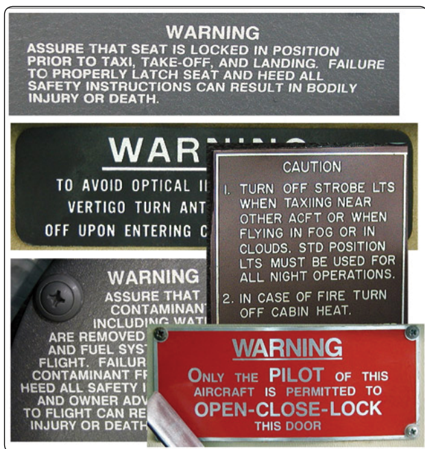
Figure 9-5. Placards are used to depict aircraft limitations.
